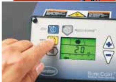
controller will automatically adjust the gun voltage to maintain the current within the preset level.
